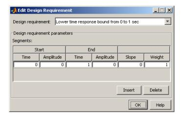
Repeat for the upper constraint, moving the constraint edge so that it begins at 0, ends at 1, and has a magnitude of 12e5. See the online documentation for more information on the Edit Design Requirement dialog box.
