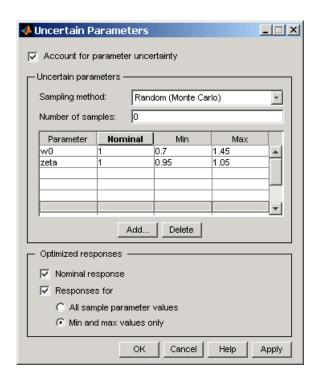
In this example, the sampling method for uncertainty is Random (Monte Carlo). The other choice is Grid in which case you would enter a vector of sample values for each parameter instead of minimum and maximum values. The number of samples indicates how many parameter value combinations to use other than the nominal, minimum, and maximum values.
