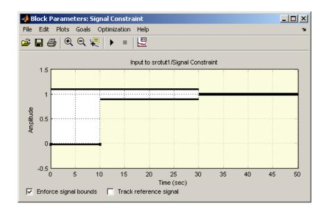
Alternatively, you could set the signal constraints using the Desired Response dialog box by selecting **Goals > Desired Response** from the Signal Constraint window. For more information on setting signal constraints, see the online documentation.
