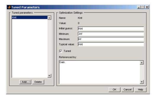
To display the optimization settings for this parameter, click Kint in the **Tuned parameters** list. The settings appear under **Optimization settings** on the right. To constrain Kint to be positive, enter **0** as the **Minimum** value. For more information on the various tuned parameter settings, see the online documentation.
