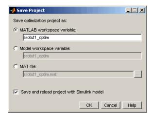
You can save the project to either a MATLAB workspace variable, model workspace variable, or a MAT-file. By selecting the **Save and reload project with Simulink model** check box, the project will automatically reload when you reopen the model. If the model cannot find the saved project when you reopen it, it gives a warning.
