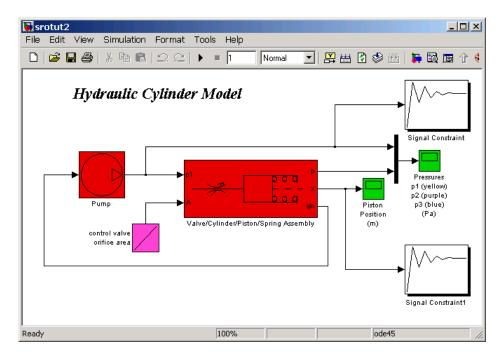
Notice that the system contains two Signal Constraint blocks. These blocks define constraints on the piston position and pump pressure signals. You can constrain multiple responses including responses within subsystems of your model. For each signal that you want to constrain, you need to attach a Signal Constraint block. Within each Signal Constraint block, set constraint bounds and/or reference signals for each signal. The tuned and uncertain parameters,
