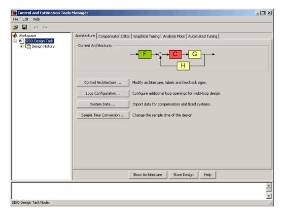
The Control and Estimation Tools Manager is a graphical environment for managing and performing tasks such as designing SISO systems. The SISO Design Task node contains five panels that perform actions related to designing SISO control systems. For more information, see "Using the SISO
