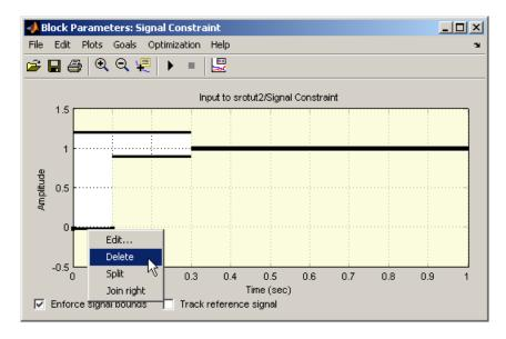
Repeat for one additional lower segment and one upper segment. The figure window should now look something like that in the following figure. Note that the thick black constraint line is actually two constraint edges positioned very close to each other.
