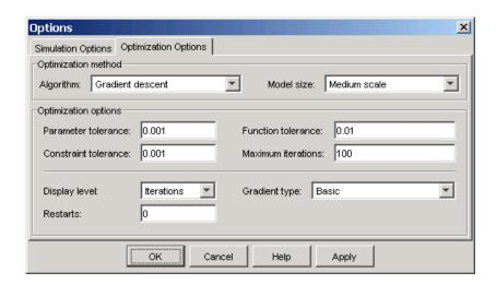
To run the optimization, select **Optimization > Start** or click the **Start** button on the toolbar in the Signal Constraint window. The results, shown next, are similar to the previous ones when only constraint bounds were used.
