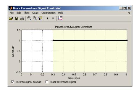
Reposition the constraint bound segments using the Edit Design Requirement dialog box. To move the lower constraint, right-click anywhere on the lower constraint segment and select **Edit** from the menu. Within the Edit Design Requirement dialog box, enter the start and end time of the constraint edge (0 and 1 respectively) as well as the amplitude of the constraint edge (since it should lie flat, both ends have the same magnitude of 0).
