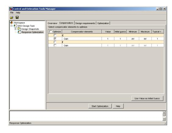
**Note** Compensator elements or parameters cannot have uncertainty when used with frequency-domain based response optimization.
