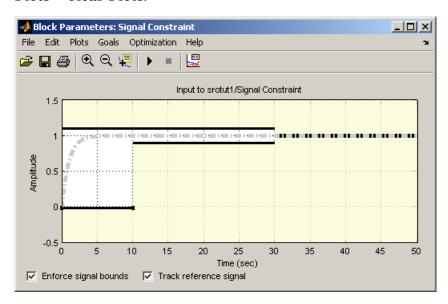
Before running the optimization, change the function tolerance to 0.01 within the Options dialog box. This ensures that the new objective function meets the imposed tolerances. To do this, open the Options dialog box by selecting **Optimization > Optimization Options** from the menu in the Signal Constraint window and then change the **Function tolerance** value to 0.01 within the **Optimization Options** pane of the Options dialog box, as shown in the following figure.
