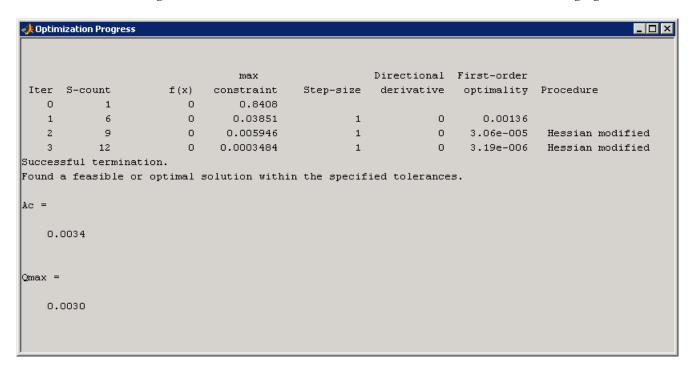
The Optimization Progress window shows the new optimized parameter values of  $0.0034~\text{m}^2$  for the cross-sectional area of the piston, and  $0.0030~\text{m}^3/\text{s}$  for the pump flow rate. These values are also changed within the MATLAB workspace.
